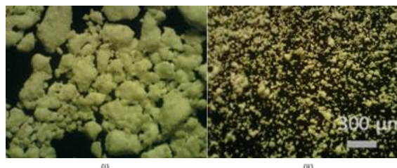
Figure 9 – MSs with 60% of the pre-hydrolysate mass, before (i) and after (ii) drying. Bar scale = 300 µm.
